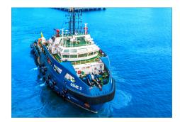
Year - 2016 Accommodation - 20 Pax Deck Area - 170 sq.m Deck Strength - 5 T/M<sup>2</sup> Draft - 4.3m Bollard Pull - 72.2T DP1
