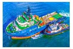
Year - 2016 Accommodation - 48 Pax Deck Area - 450 sq.m Deck Strength - 7 T/M<sup>2</sup> Draft - 4.5m Bollard Pull - 82.2T Hybrid DP2
