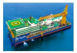
Year - 2015 Accommodation - 402 Pax Deck Area - 1500 sq.m Deck Strength - 15T/m<sup>2</sup> Draft - 3.5m Crane Capacity - 300T 10-Point Mooring System Heavy Lift & Pipe lay Capabilities
